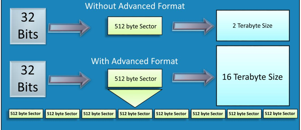
6:44 – To improve support for larger drives with older hardware, Advanced Format was developed and is available for use with all hard drives manufactured since 2011. This potentially allows hard disks larger than 2 Terabytes to be used on older hardware and software that does not support GPT.
