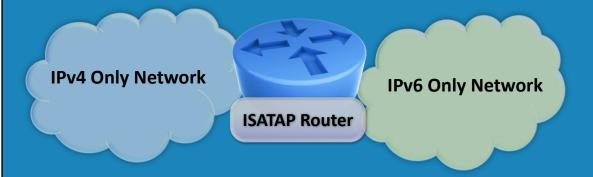
05:15 – ISATAP stands for Intra-site Automatic Tunnel Address Protocol. The main takeaway from the name is the "Intra" in Intra-site which stands for internal. ISATAP is designed to work within a site or internal network. This means it is not used for public communications across the Internet. An easy rule when encountering ISATAP on an exam is to eliminate any options that involve external communications.
