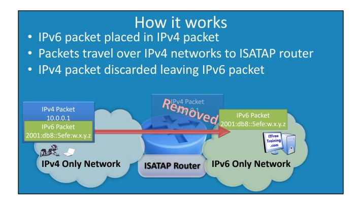
2:10 – In order to understand, the ISATAP transition technology, we'll take a look at a different example. ISATAP utilizes tunneling to communicate data from the IPv4 host to the ISATAP router. This essentially states that an IPv6 packet will be embedded, or placed, within an IPv4 packet.
