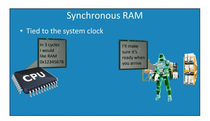
0:1:23 By contrast, synchronous RAM is tied to the system clock. With synchronous RAM, the CPU will once again ask for the contents of RAM. Unlike before, the CPU will now tell the RAM that it will be back after a certain number of cycles for the contents of the RAM.
