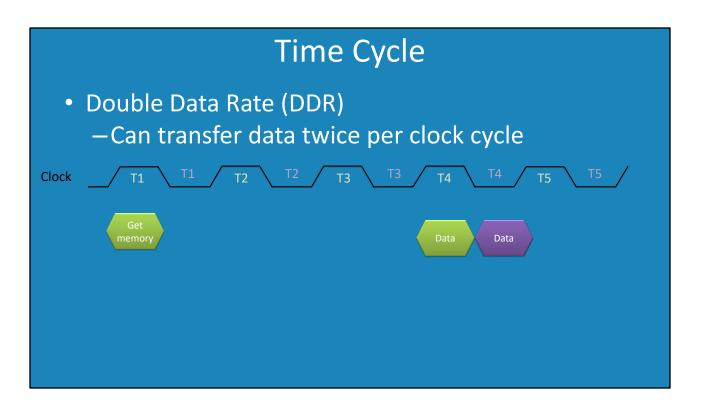
0:2:13 To understand synchronous memory better, consider the following time cycle. The CPU generates the time cycle. The memory module receives the time cycle and synchronizes its operations to this time cycle.
