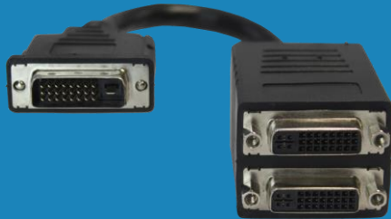
Passive cable Effectively divides signal in half
