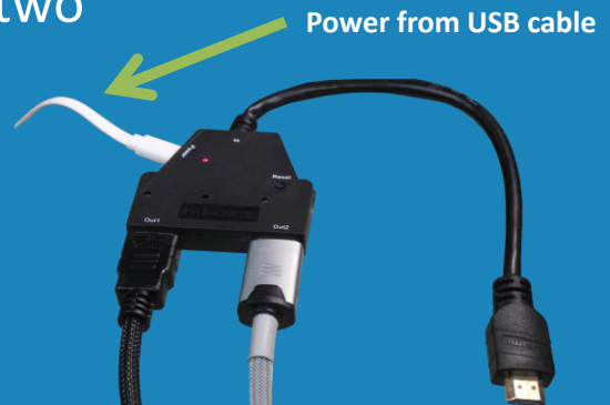
Active cable Recreates or boosts signal May require additional power
