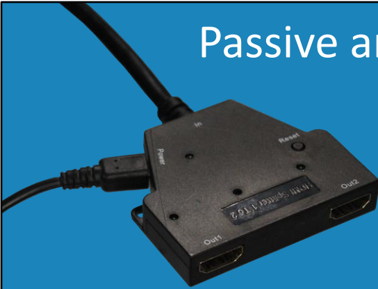
HDMI Splitter Powered by USB Signal not reduced by splitting
