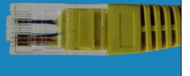
1:00 Let's consider a standard network cable, which we would in IT refer to as RJ45. This particular cable, therefore, meets the standard called RJ45. This is because, in order to meet the standard, it needs to have eight positions. A position simply means somewhere a connector can be mounted to. The next requirement it needs in order to meet the standard is that it needs to have eight wires or four pairs of wires. You can see that this connector has this and, thus, meets the standard for RJ45.
