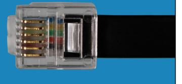
2:40 The next connection that I will look at is the RJ11 connection. To be technically correct, this connector has six positions and two wires or one pair. This connector is often use to connect telephones.
