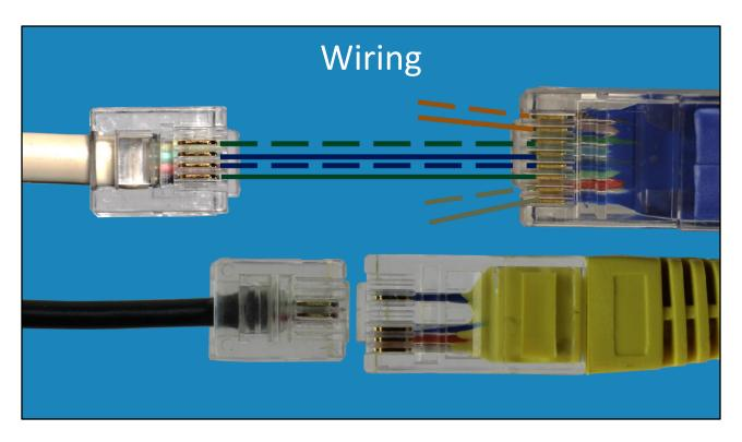
6:12 To understand how compatibility is achieved, let's consider the wiring of the cable. Before networking became widespread, the telephone was commonplace. For networking to be compatible with telephones, the plug needed to support one or two pairs of wires. For telephones, the inner wires are the first pair and the outer wires are the second pair.
