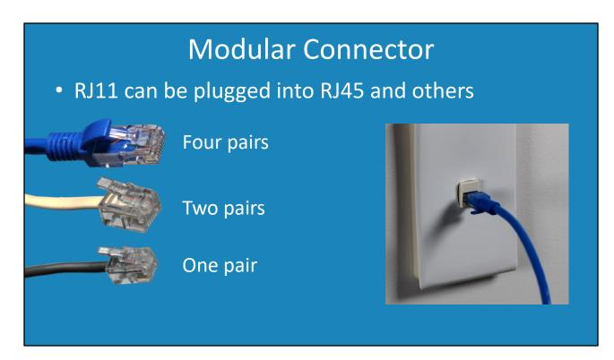
4:18 The registered jack is also referred to as the modular connector. In fact, it was called a modular connector before it was given the name registered jack. It is given this name because multiple connectors can be put into the same plug. For example, RJ11 and other connectors can be plugged into an RJ45 plug.
