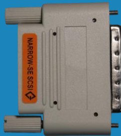
SCSI Terminator Plugged into last device
