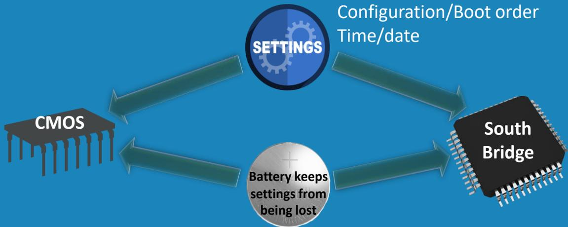
8:46 One common misconception I would like to bring up, is the difference between CMOS and BIOS. CMOS stands for Complementary metal-oxide semiconductor. In the old days of computing the CMOS was a separate chip on the motherboard. Nowadays the functions of CMOS have been integrated into the south bridge, so that on modern motherboards CMOS is not a separate chip.
