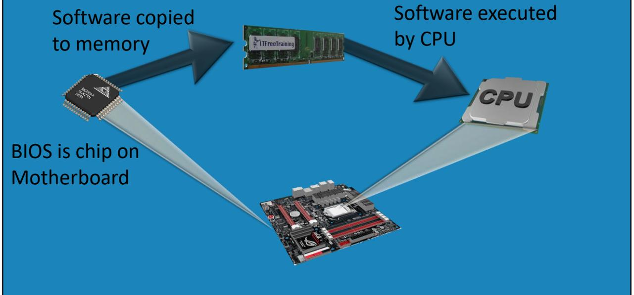
1:56 The BIOS is essentially a microchip on the motherboard. This is also often referred to as firmware. Older BIOS chips use Electrically Erasable Programming Read-Only memory called EEPROM, whereas modern BIOS uses flash RAM. This allows the code in the BIOS to be updated, but the code on the BIOS cannot be directly run from the chip itself.
