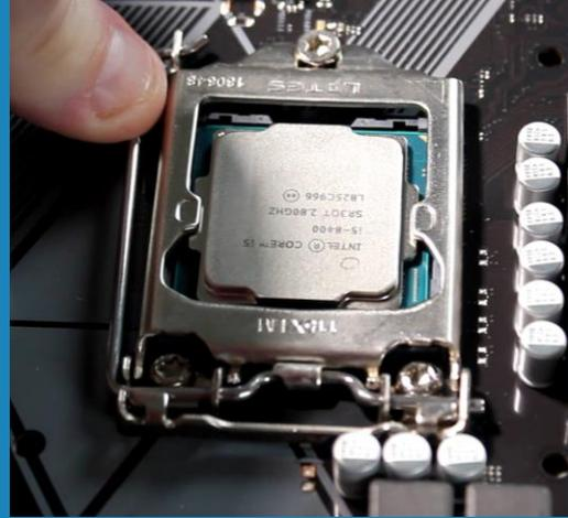
17:31 Next, I will look at the current sockets being used on the market. The current sockets being used are LGA or Land Grid Array. The big difference is that the pins are not in the CPU but on the motherboard. Having the pins on the chip increases the chance they may be bent or damaged when handling the CPU. This change was made to reduce the risk of damaging the CPU when installing or handling it.
