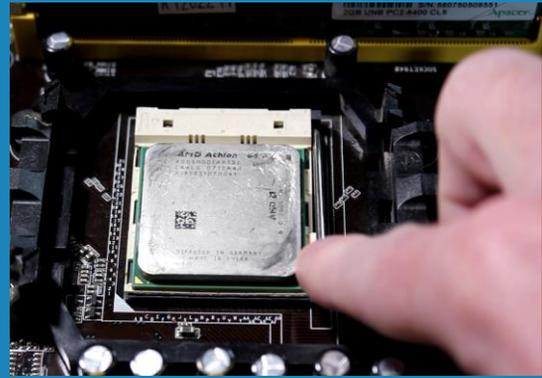
15:54 With the change from slot back to sockets, let's now have a closer look at the socket. The socket we will look at is the PGA-ZIF socket. This socket dominated the market until 2004. PGA stands for Pin Grid Array. This essentially means that the pins are mounted on the CPU and the socket contains pin holes.
