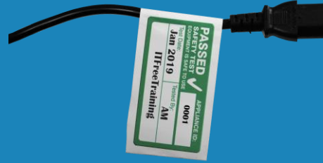
Cable tested and tagged
