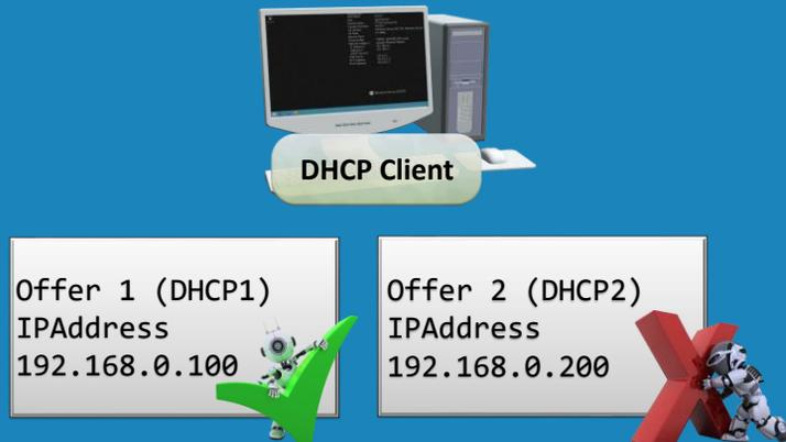
The next step is that a DHCP Request message is sent to the DHCP server. However, let's consider that the DHCP client in this example has two DHCP offers so, which one does it accept? Generally speaking, the device will accept the first offer. The second offer will be discarded. If there were any other offers, they would also be discarded.
