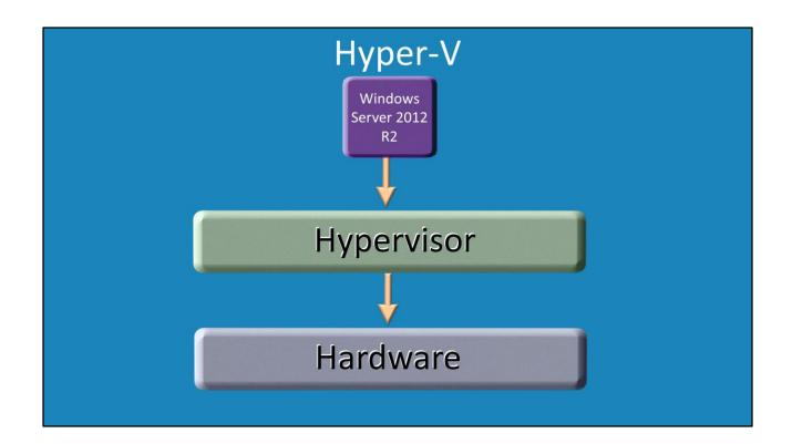
When Hyper-V is installed, the HAL is replaced by a Hypervisor and the operating system and virtual machines access the hardware through the hypervisor. So essentially the hypervisor is a HAL with additional features required for virtual machines.
