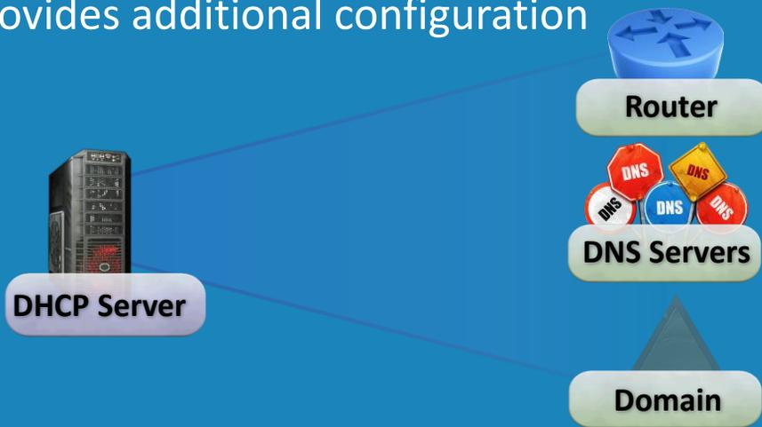
0:12 A DHCP server can be configured to provide additional configuration for a device on the network. Without additional configuration, the device only has an IP Address and subnet mask, not enough configuration to allow it to communicate on a network and find other resources.
