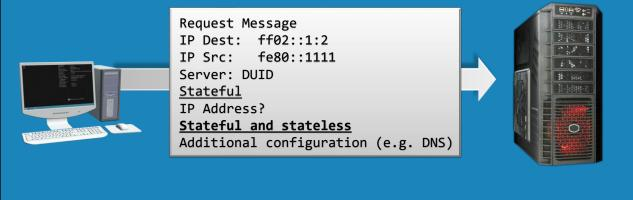
12:33 The next step is for the device to send a Request message to a DHCP server. Just to recap, the Request message is only sent when stateful mode is used, or stateless mode is used with the Other Configuration bit set to one.
