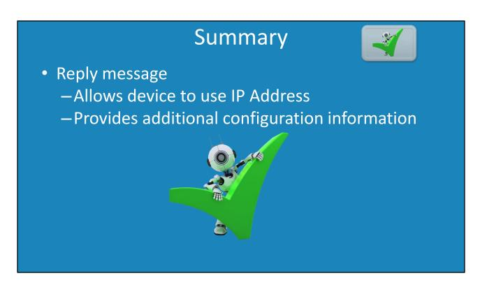
19:16 The last message that is sent is the Reply message. This message informs the device that it may use the IP Address when stateful is being used. The Reply message also contains any additional network configuration for the device to use. For example, DNS servers.
