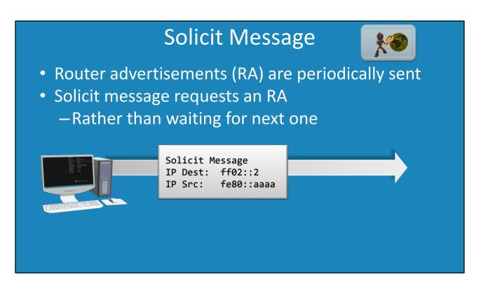
4:37 On an IPv6 network, router advertisements are periodically sent over the network. As we will see later in the video, these messages are used to create a valid IP Address that can be used to access local and remote networks. If the device does not wish to wait for the next router advertisement message, the device can send a solicit message which requests a router advertisement message to be sent.
