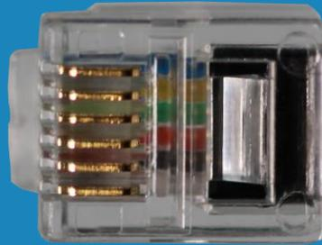
2:40 The next connection that I will look at is the RJ11 connection. To be technically correct, this connector has six positions and two wires or one pair. This connector is often use to connect telephones.
