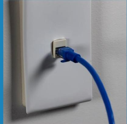
4:18 The registered jack is also referred to as the modular connector. In fact, it was called a modular connector before it was given the name registered jack. It is given this name because multiple connectors can be put into the same plug. For example, RJ11 and other connectors can be plugged into an RJ45 plug.
