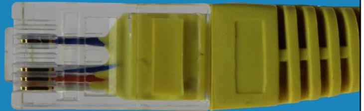
1:00 Let's consider a standard network cable, which we would in IT refer to as RJ45. This particular cable, therefore, meets the standard called RJ45. This is because, in order to meet the standard, it needs to have eight positions. A position simply means somewhere a connector can be mounted to. The next requirement it needs in order to meet the standard is that it needs to have eight wires or four pairs of wires. You can see that this connector has this and, thus, meets the standard for RJ45.
