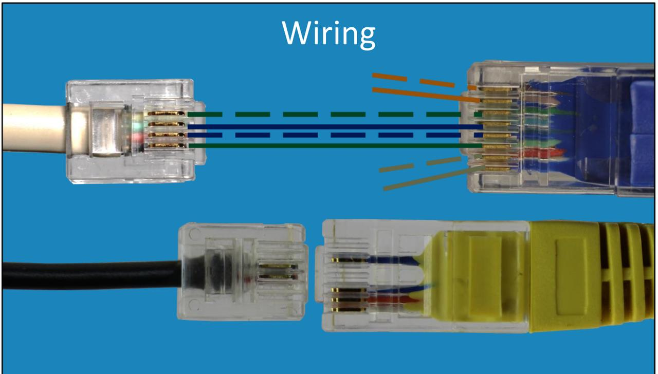
6:12 To understand how compatibility is achieved, let's consider the wiring of the cable. Before networking became widespread, the telephone was commonplace. For networking to be compatible with telephones, the plug needed to support one or two pairs of wires. For telephones, the inner wires are the first pair and the outer wires are the second pair.
