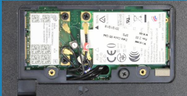
Two MiniPCle cards with connectors inside a laptop
