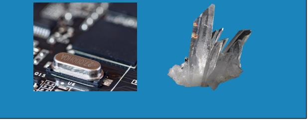
1:14 On your motherboard there will be one or more crystal oscillators. They come in different shapes and sizes, but with computers they generally tend to be a rectangular component with rounded corners soldered onto the motherboard.
